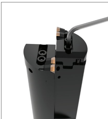
Step 5: Tighten the mounting screws on the cartridge to 15-19 Nm (11-14 ft-lbf).
